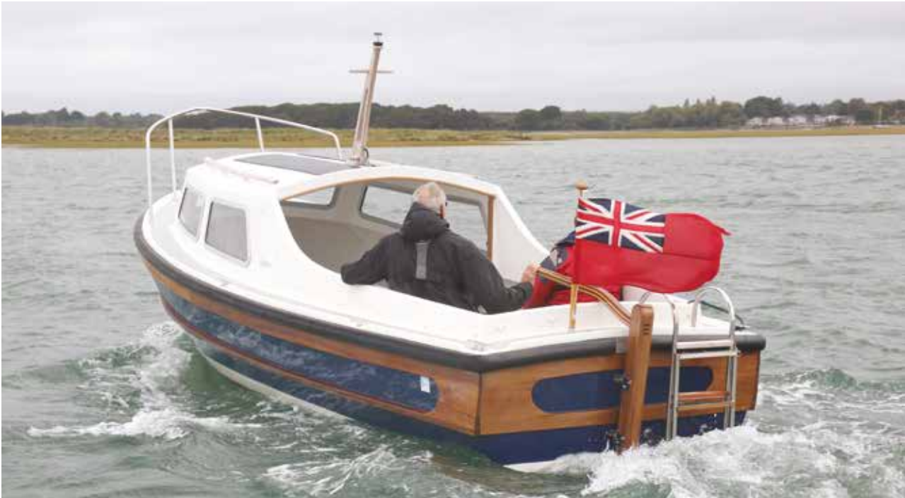
Above: The Classic Cabin version tested had one pod motor and a single battery which delivered a run time of 8 hours at 4 knots. Facing page: The Workboat version, with twin pods and two batteries, gave the same figures but with more power in reserve.
