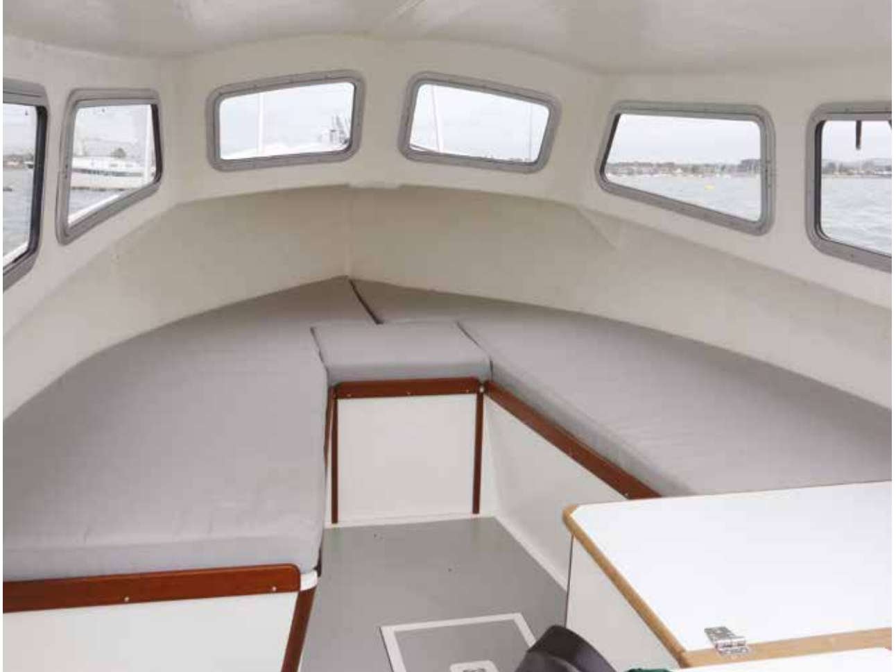
Facing page: The Classic Cabin version of today's Nelson 18. The new range comes with the options of diesel or electric propulsion. Above: The Classic's cabin has two berths with a chemical toilet hidden between them. The port berth can house a refrigerator.
